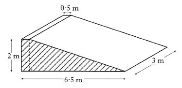
Find the volume of concrete required to make the ramp.
