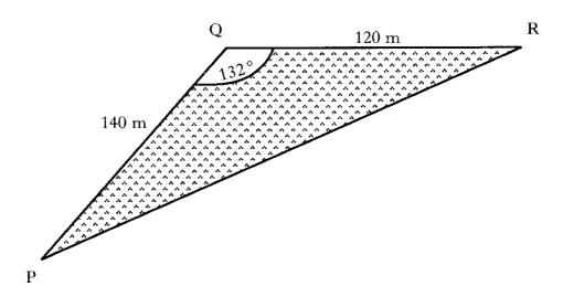
PQ = 140 metres, QR = 120 metres and angle PQR =  $132^{\circ}$ . Calculate the length of PR.
