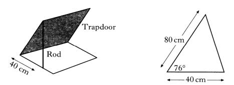
The rod is attached to a corner of the trapdoor and placed 40 centimetres along the edge of the opening.
