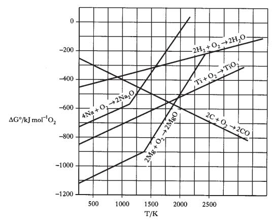
The reduction of  ${\rm TiO_2}$  to Ti is thermodynamically feasible at 1500 K using
